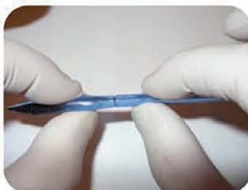
Separating head of device from handle
